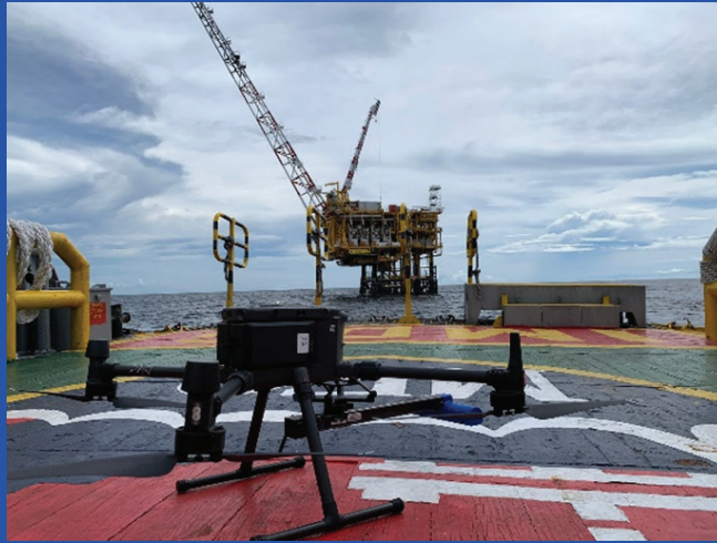
"Sniffer" sensor mounted on a drone operating over an offshore platform.
