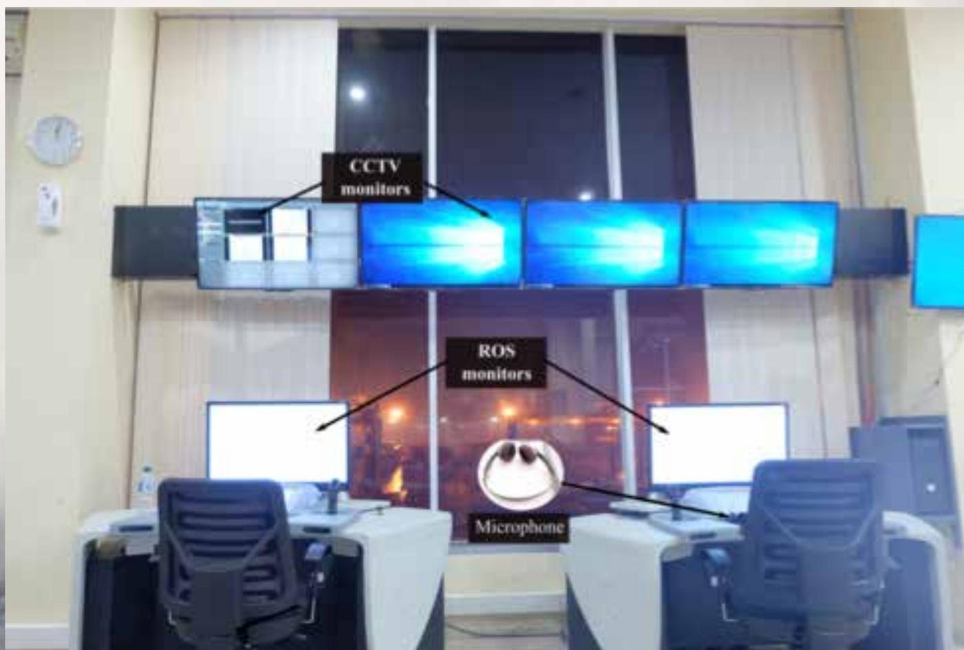
Figure 2 Remote operator station (ROS) for remote-operated crane operation
