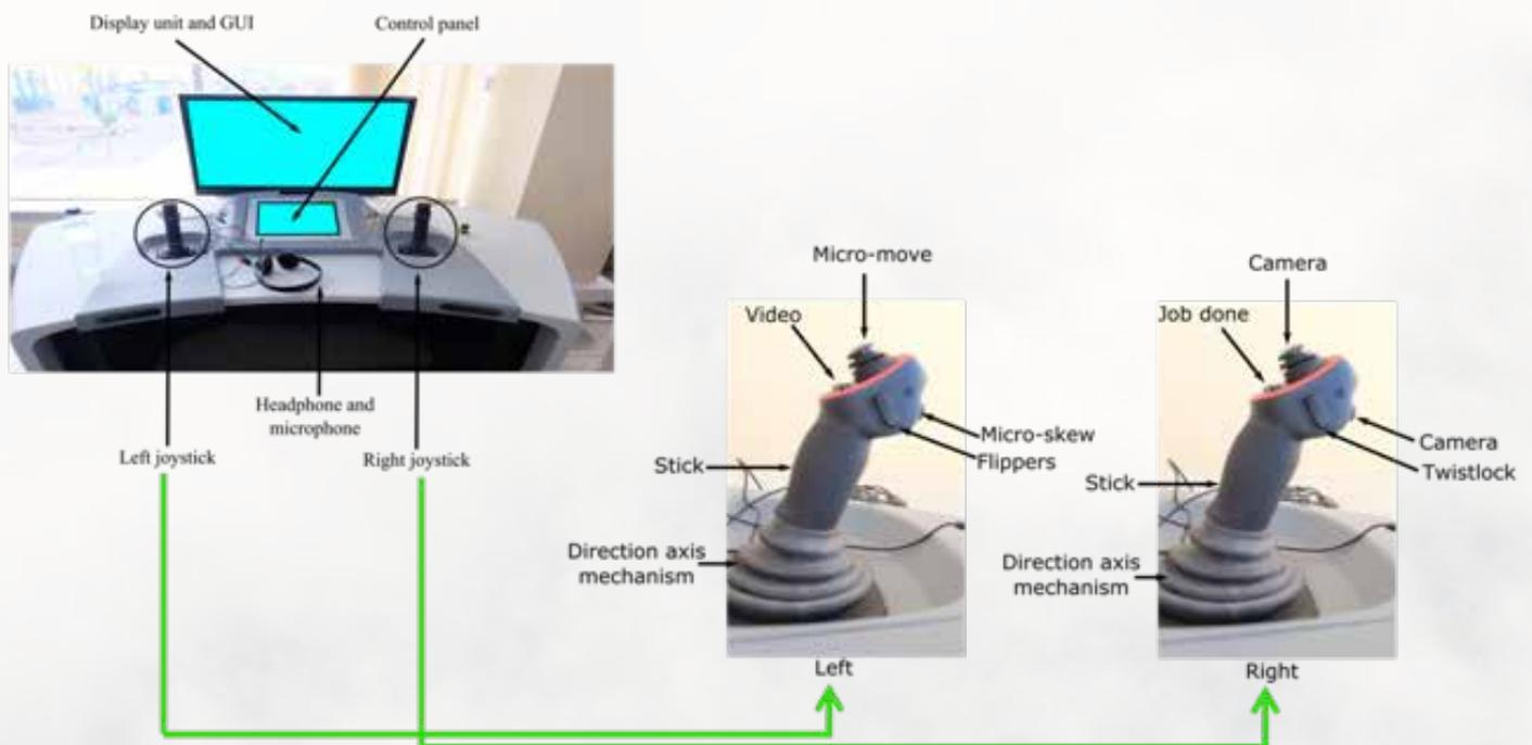
Figure 3 Joystick as remote-operated control and handling interface
